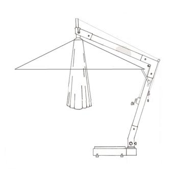
ALWAYS USE THE LOCKING ARM WHEN THE WIND GOES ABOVE 10mph/15kph AND DO NOT HAVE THE CANOPY TILTED IF THE WIND IS ABOVE 10mph/15kph.
